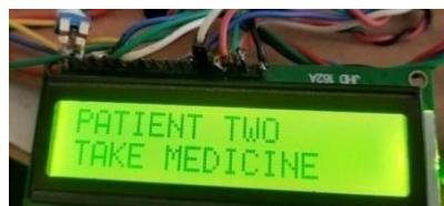
Figure 14: LCD Display of Medicine / Tablet Dispensing
